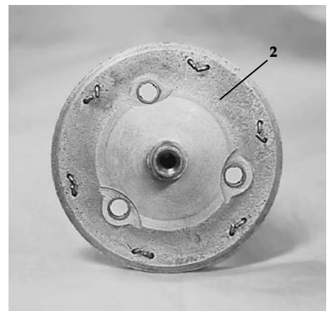
Photo 12: Back side of inner driving plate (2) showing staples holding on servo liner.
