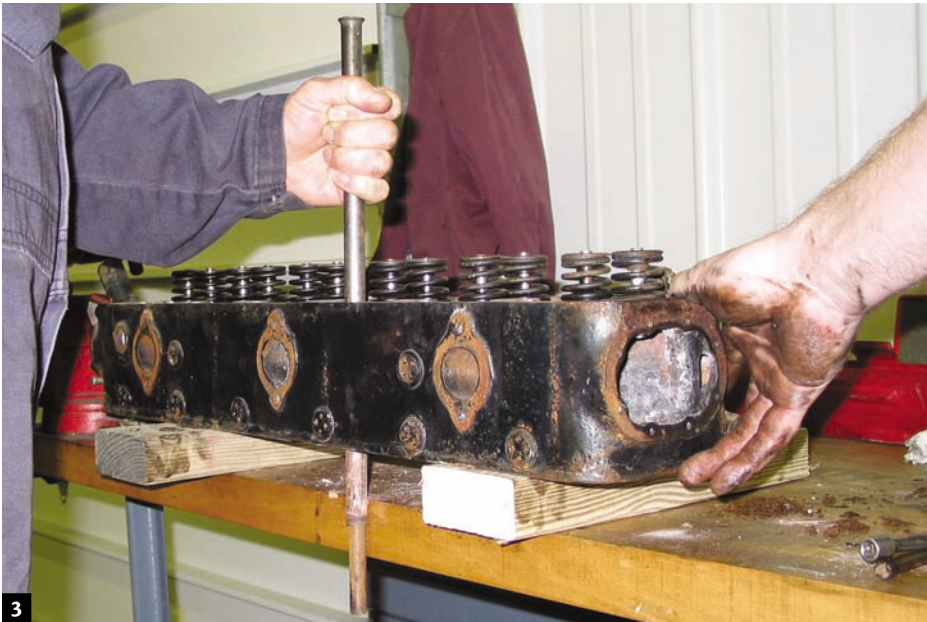
3 Copper tubes in the head are removed with a special stepped punch. It is recommended to remove the tubes in the head and block to facilitate more thorough cleaning of silt and rust to improve water circulation after an engine rebuild.
