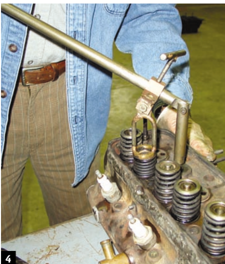
4 Shop-made tool to compress valve springs. The end is threaded \frac{5}{16} " BSF and screws on to the rocker arm bolts. The handle has a sliding arm to center the tool over each valve spring. This design allows you to remove the two valve springs closest to each rocker arm bolt.
