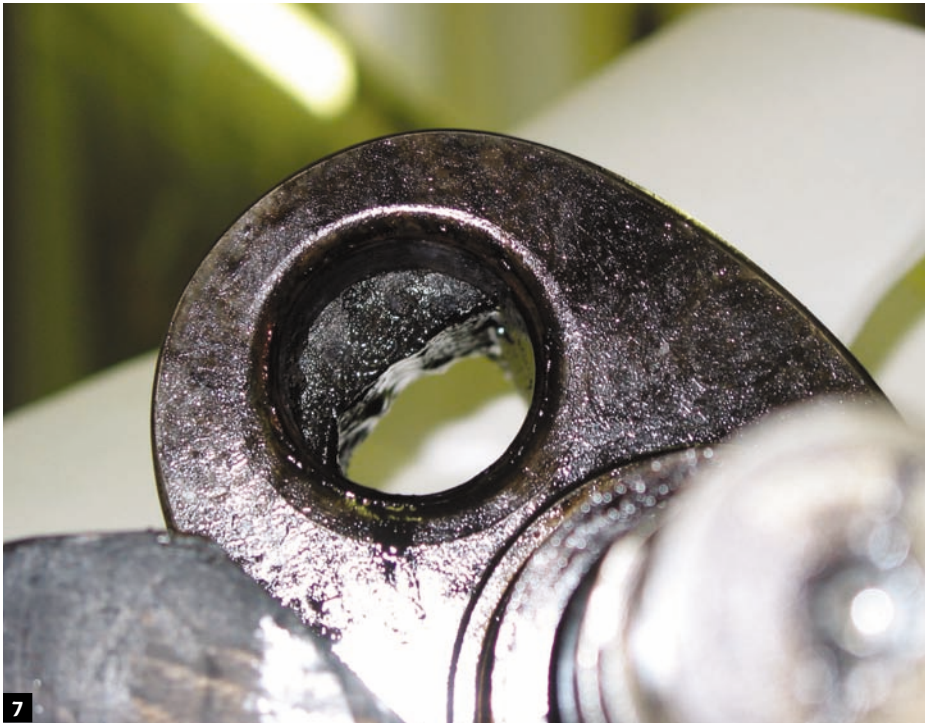
The crankshaft has hollow journals that fill with oily sludge as a result of the centrifugal-like action of the spinning crankshaft. Aluminum plugs seal the ends of the journals and are held in place by through-bolts. The plugs should be removed and the sludge cleaned out so that oil flows freely to the big ends of the connecting rods. Note build-up of sludge in journal.
