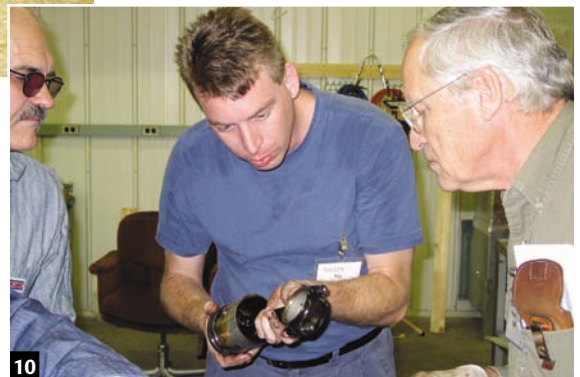
The connecting rod has an external oil line that is soldered at the top and bottom of the rod. The solder joints are subject to coming loose and should be pressure tested to insure they do not leak. You can fish a piece of piano wire down each oil line to insure it is clear. The integrity of the oil line is important since it is the sole source of lubrication to the small end of the connecting rods.
