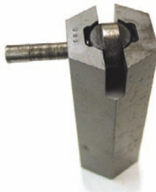
14 Shop-made tool to remove the pin in the cam roller bearing. The hex stock was bored out to accept the cam roller bearing and slotted to hold the wheel in place. A cross-drilled hole allows a punch to be centered on the wheel for removal of the pin.
