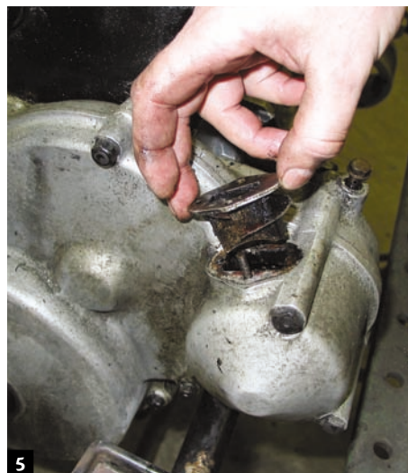
5 Before removing the front timing cover, remove the upper and lower dynamo brakes that are held in place by two nuts. The "bearing" surface of the dynamo brakes is made of lignum vitae, a very hard, dense wood that is often used for propeller shaft bearings in boats.
