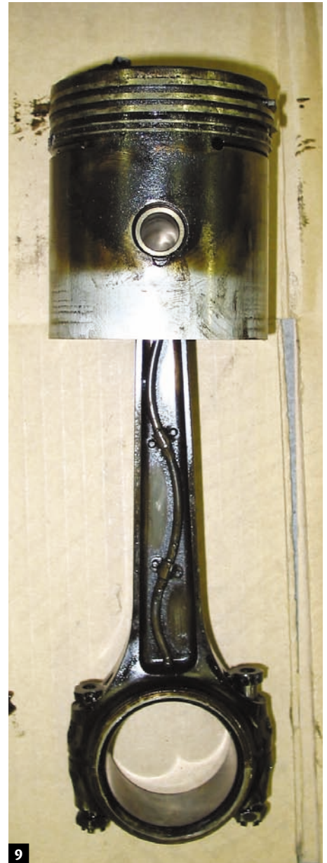
The connecting rod has an external oil line that is soldered at the top and bottom of the rod. The solder joints are subject to coming loose and should be pressure tested to insure they do not leak. You can fish a piece of piano wire down each oil line to insure it is clear. The integrity of the oil line is important since it is the sole source of lubrication to the small end of the connecting rods.
