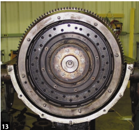
13 The flywheel bolts are peened over or center-punched to secure them. You have to grind off the bolt edges to remove the nuts. Be sure and use new bolts on the rebuild.
