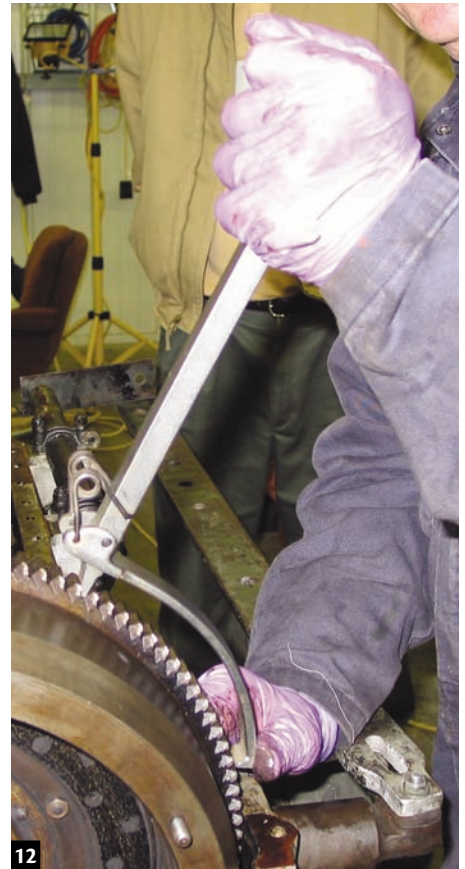
12 Snap-On makes a generic flywheel tool (A144) that fits the small horsepower flywheel. It can be used to turn the flywheel or hold it in place to remove the flywheel bolts.
