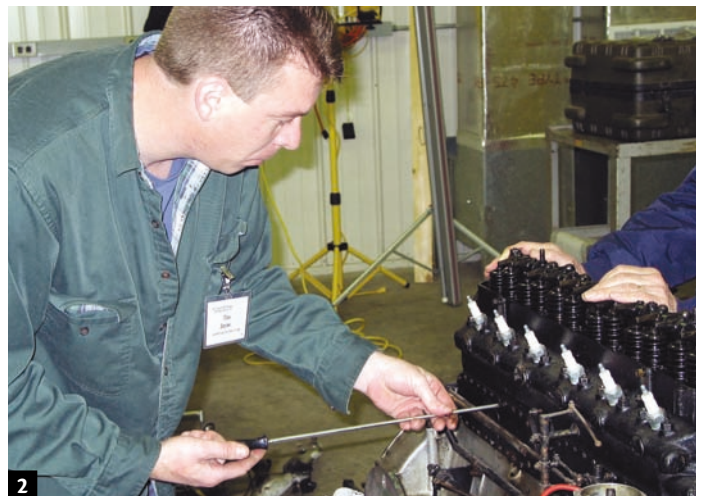
2 Tim Jayne uses a long screwdriver with tip ground to exactly fit the 2BA screws that hold on the side plates on the block.
