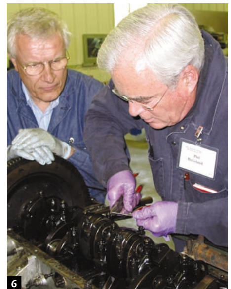
6 Peter Sedmihradsky (ONT) and Phil Birkeland (WA) work on removing the numerous cotter pins securing the castellated nuts on bearing caps.
