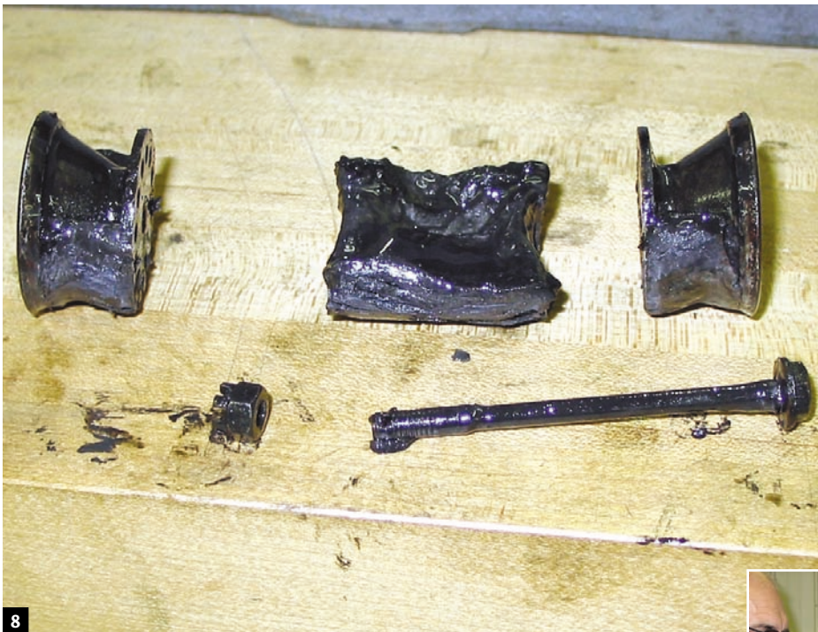
Aluminum sludge trap seals showing build-up of oil sludge and plug of sludge (middle) removed from journal.
