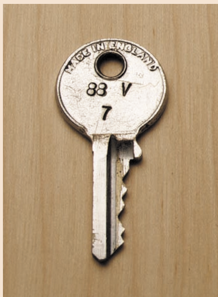
Pre-war Yale key showing characteristic key code (88 V 7). This number corresponds to the key code stamped on the barrel of the ignition switch located behind the dash and is also referenced in the chassis cards.
