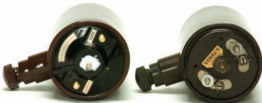
Under the mushroom-shaped cap, the terminals of the River Carriage coil are clearly marked for wiring. Note the epoxy seal around the inner edge to seal out moisture. By comparison, the cap on the original coil is not sealed and was subject to moisture degradation.
