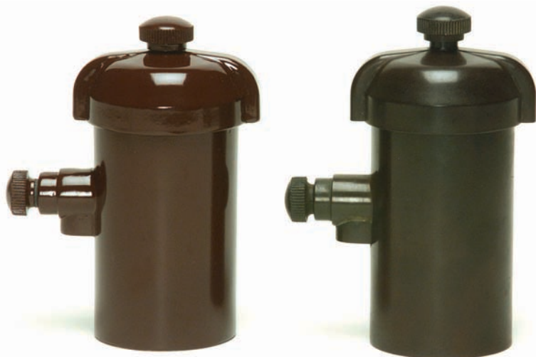
The River Carriage coil (left) is made of high-impact plastic and includes a high-efficiency electrical core that is epoxy sealed. An original coil (right) is shown for comparison.
