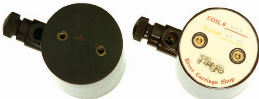
The base of the River Carriage coil is stamped with a serial number and test date. The base includes captive nuts for mounting the same as the original coil (left).
