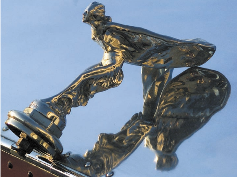
The Swift Method achieves a micro-finish on aluminum with high gloss, definition and depth as evidenced by the reflection of the Flying Lady mascot in 3AU's bonnet, the author's 1924 Silver Ghost.
