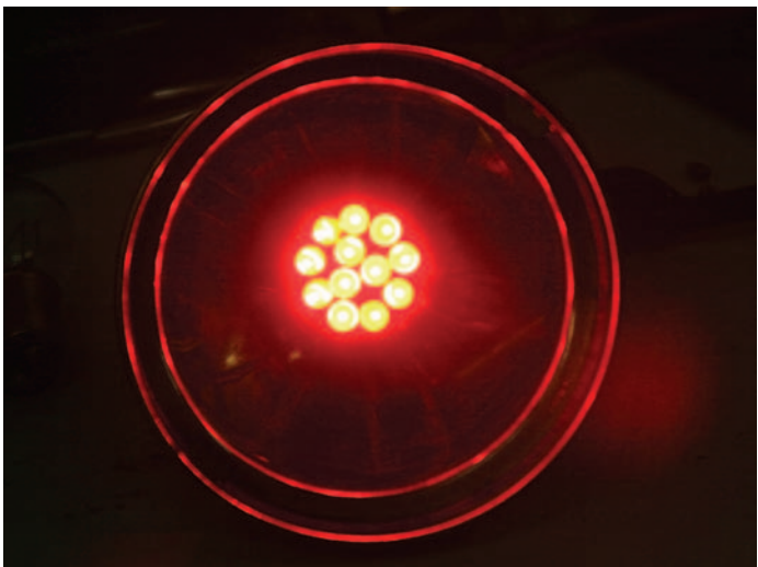
The $5 LED has 12 individual LEDs that are all located on its tip and that results in a quarter-sized point of light. Very little of the light is picked up in the mirrored reflector of the prewar tail lights since the LED's light is very directional.
