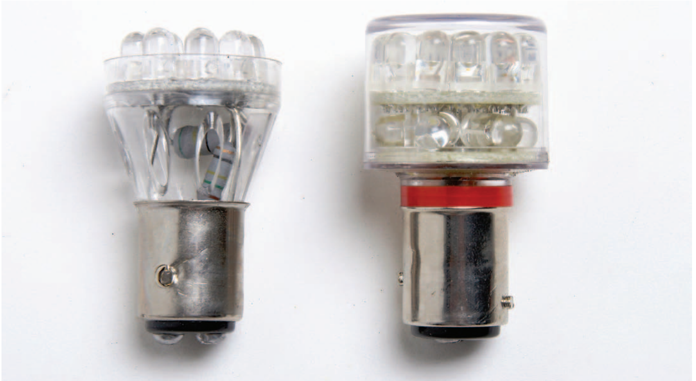
LED bulbs can vary widely. The 12 segment LED bulb (left) sells for about $5 and is widely available at automotive stores. The 24 segment LED bulb (right) is made by Ledtronics ( www.ledtronics.com ) and sells for about $25. The Ledtronics bulb includes side- and top-facing LEDs that provide brighter and more even illumination in many reflector assemblies than designs with all the LEDs pointed in one direction.
